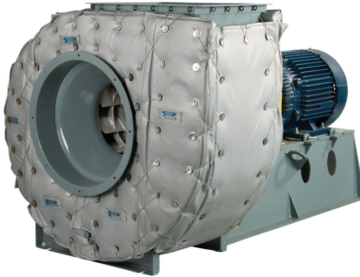
Arrangement 8 (left) direct drive fan. Fan shown includes an acoustical blanket to reduce radiated noise.
